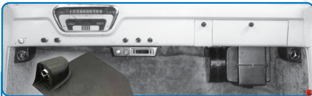
Electronic Control Technology Electronic Bypass Heater Valve & Defrost Servo Motor
