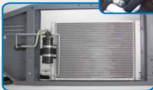
51-6601 Condenser Assembly Includes brackets, drier & custom tube set
