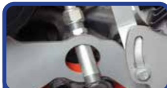
91-1001 O-ring heater fitting shown on Small Block Chevrolet engine with long water pump. Excellent for additional clearance of heater nipple through aftermarket brackets.
